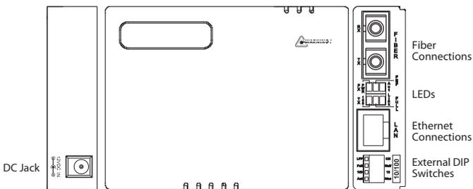
Figure #2. FMC-10/100-AC, FMC-10/100-DC
